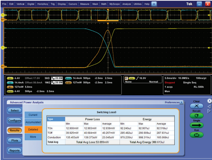
Figure 5. DPOPWR automated switching loss measurement.
