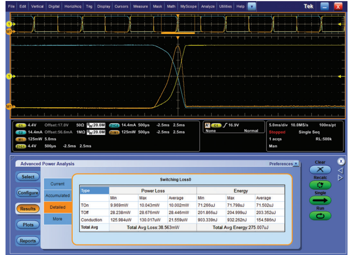
Figure 8. DPOPOWER automated switching loss measurement, showing significant improvement.
