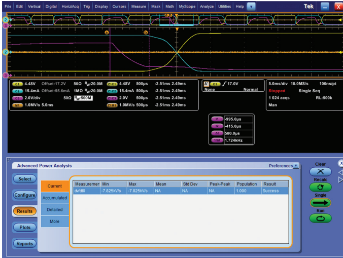
Figure 7. Automated slew rate measurement on MOSFET gate.
