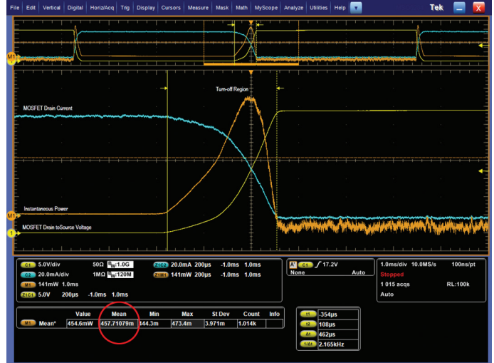
Figure 4. Gated automatic measurement of turn-off power loss in a MOSFET switch.
