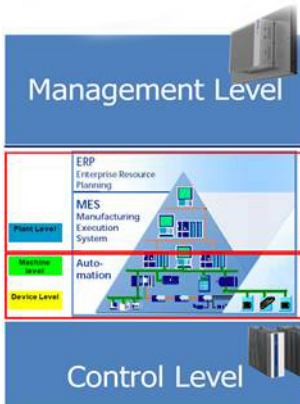
Figure 4 - An IPC can act as the bridge from plant floor automation systems to higher level computing platforms such as an ERP system or an MES.
