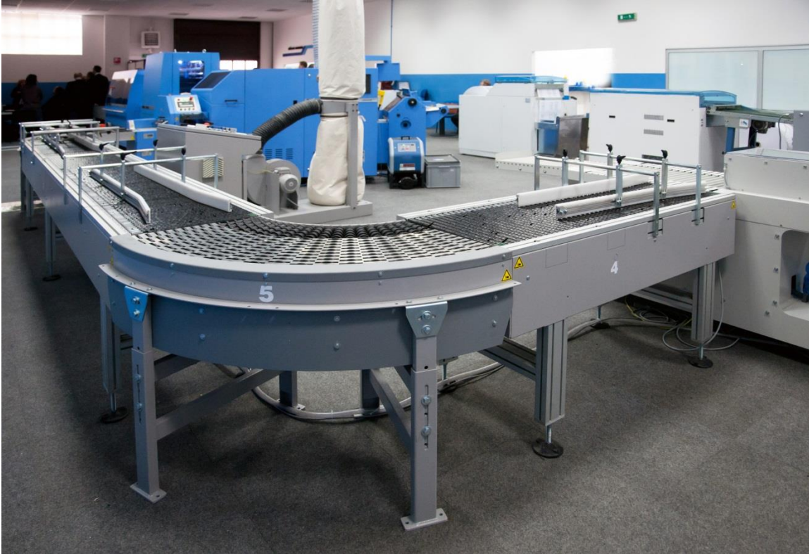
Figure 3 - Machines like this one can be retrofitted with wireless I/O modules to bring them into the IoT world, allowing for quick and simple monitoring via any web-connected PC or mobile device.
